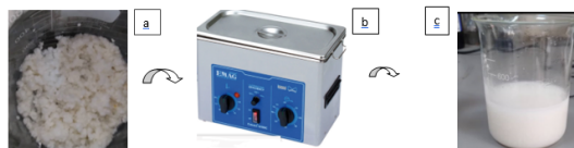
Figure 1: Hydrolysis method of Alfa fiber; (a): pretreated/ bleach fiber; (b): Ultrasonic cleaner; (c): solution of Alfa Nanofiber
